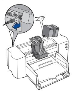
d. Remove the print cartridges and place them on their sides on a scrap piece of paper.
