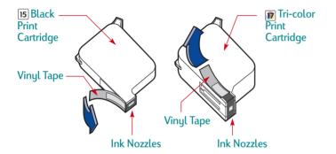
5 For each print cartridge, lift the cradle latch inside the printer. With the copper electrical contacts toward the rear of the printer and the print cartridge held vertically, push the print cartridge firmly down into the cradle.
