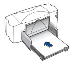
5 Slide both paper adjusters to fit snugly against the paper's edges. Make sure the paper lies flat in the tray and that the paper fits under the tab of the paper-length adjuster.
