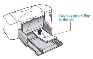
4 Slide the paper adjusters so that they fit snugly against the edges of the envelopes.
