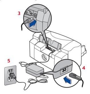
**Note:** Always use the Power  $\circlearrowleft$  button on the front of the printer to turn the printer on and off. Using a power strip, surge protector or a wall outlet switch to turn the printer on and off may cause premature failure.
