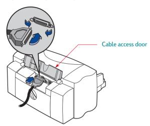
4 Plug the other end into the computer, and tighten the screws.
