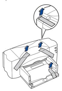
2 Open the top cover. Remove both pieces of plastic packing material from the inside of the printer.
