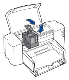
7 Close the cradle latch. You will notice some resistance when closing the latch. When the latch is fully closed, you will hear a click.
