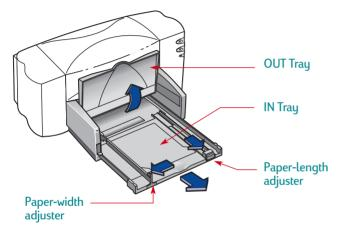
2 Remove a stack of paper from its packaging. (Make sure all the paper in the stack is the same size and type.) Tap the stack on a flat surface to even it up.
