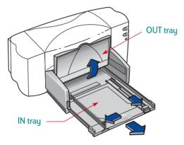
Make sure the edges of the envelopes align with the right side of the IN tray.
