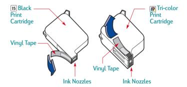
5 For each print cartridge, lift the cradle latch inside the printer. With the copper electrical contacts toward the rear of the printer and the print cartridge held vertically, push the print cartridge firmly down into the appropriate cradle.
