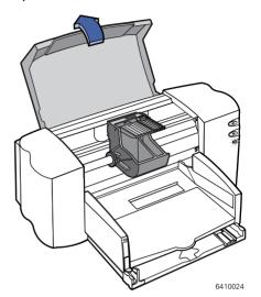
**Note:** Be sure not to touch the ink nozzles or the copper electrical contacts. Also, do NOT remove the copper strip; these are electrical contacts required for proper operation of the inkjet print cartridges.
