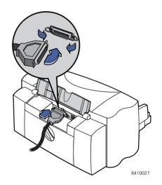
4 Plug the other end into the computer, and tighten the screws.
