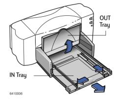
3 Put a stack of up to 15 envelopes in the printer, as shown below. (If you're using thick envelopes, you might need to reduce the number.)
