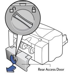
If you can't see the paper causing the jam, check to see if a label has come unglued from a label sheet while going through the printer.
