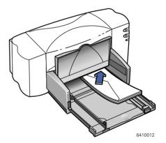
4 Slide the paper adjusters so that they fit snugly against the edges of the envelope.
