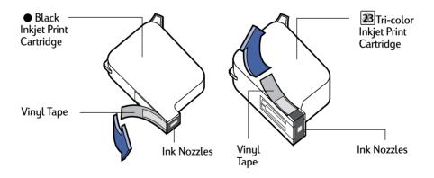
5 For each inkjet print cartridge, lift the cradle latch inside the printer. With the copper electrical contacts toward the rear of the printer and the inkjet print cartridge held vertically, push the inkjet print cartridge firmly down into the cradle.
