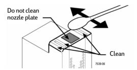
3 Clean the face and edges of the inkjet print cartridge as shown. DO NOT wipe the nozzle plate.
