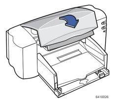
**Note:** If the Inkjet Print Cartridge light continues to blink or if the cradle doesn't move to the right side of the printer, take out both cartridges and reinsert them.
