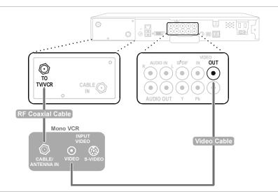
4 Connect an RF coaxial cable to the TO TV connector on the VCR and the CABLE/ANTENNA IN connector on the stereo TV:
