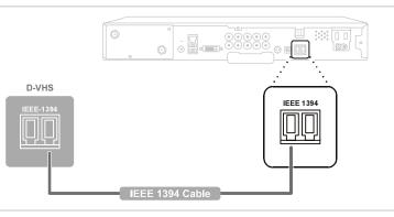
**3** Connect an IEEE 1394 cable to the **IEEE 1394** connectors on your D-VHS digital VCR and HDTV.
