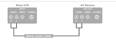
**5** Connect a stereo audio cable to the **OUTPUT AUDIO R** and L connectors on the stereo VCR and the **VCR INPUT AUDIO R** and L connectors on the A/V receiver, as shown below:
