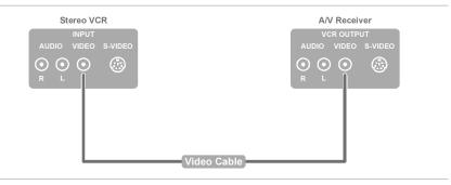
7 Connect a video cable to the **OUTPUT VIDEO** connector on the stereo VCR and the **VCR INPUT VIDEO** connector on the A/V receiver.
