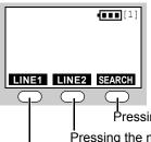
3 soft keys are used to select functions displayed directly above each key. Functions displayed above each key will change depending on the state of use.
