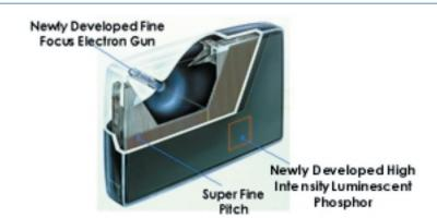
Super Fine Pitch™ CRT provides better image detail with high definition sources. The Aperture Grill was improved by making the vertical slits a finer pitch that increases the number of slits by up to 65% (16x9 base). Also improved were the High Precision Deflection Yoke, Fine Focus Electron Gun and the inclusion of higher intensity Luminescent Phosphors. The result is a more detailed image for both moving and still images, higher resolution picture quality, and better edge detail.
