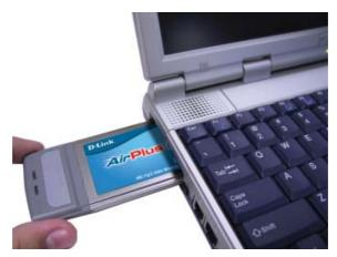
C. Gently insert the DWL-G630 into the cardbus slot in your laptop computer (as shown.)
